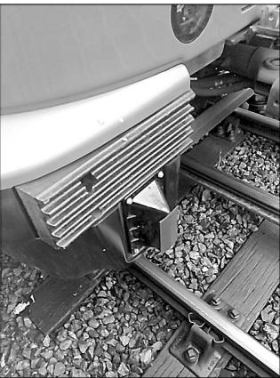
Modifications are being made to the S8 Stock. Having had problems with receiving in-cab CCTV images at some locations, it has been necessary to bring the 'plate' forward. At the time of writing, two thirds of the fleet had been modified. The above show the receiving aerials for the station CCTV cameras and positioning beacons at stations in modified form. It will be interesting to see if the S7 fleet is similarly modified.
